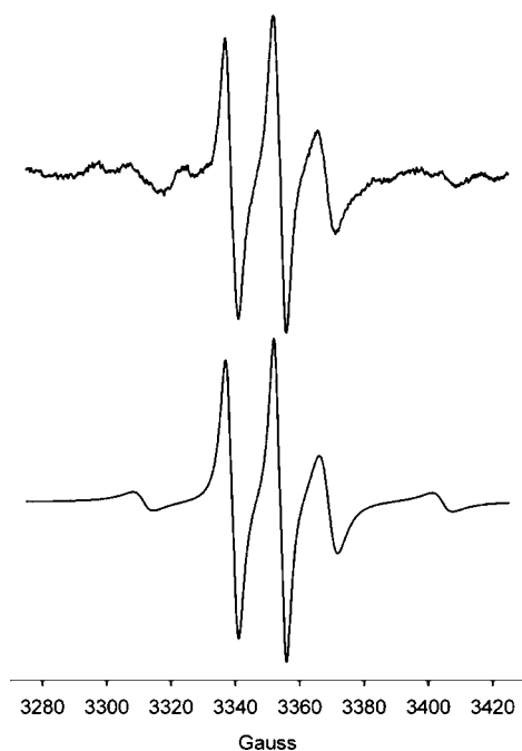
Figure 3. Experimental (top) and simulated (bottom) EPR spectra of ultrasound-treated sunflower oil.
